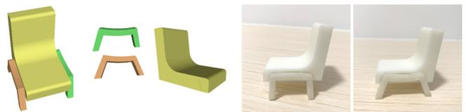
Fig. 17. An example of multi-material fabrication. The chair legs are fabricated by flexible material that can be deformed to different shape.
