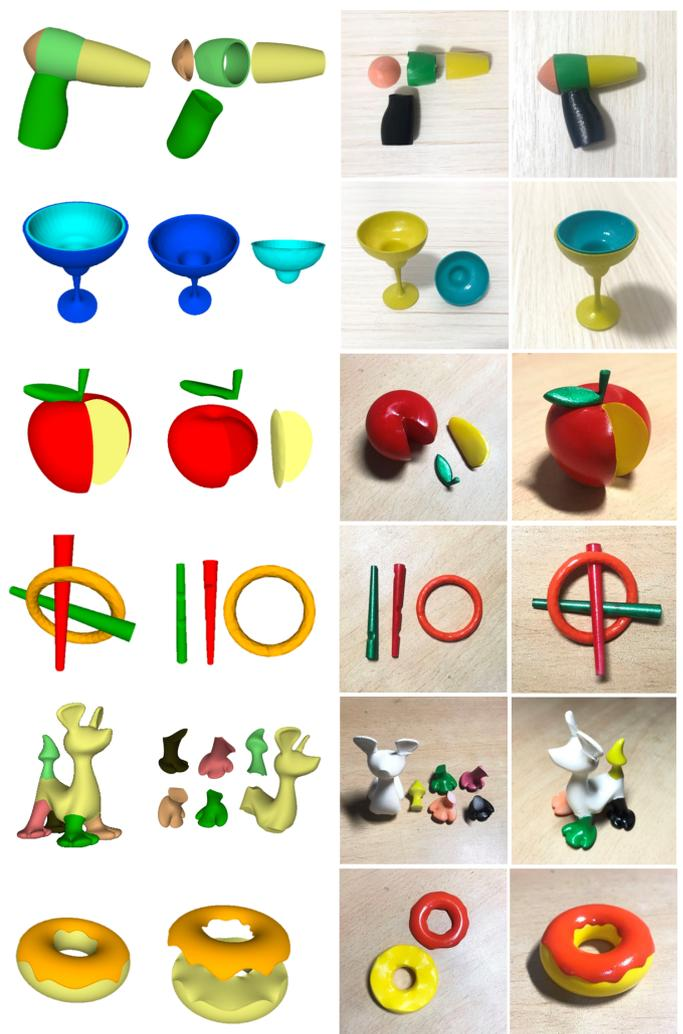
Fig. 16. Various model segmentation results using our approach and their corresponding printed objects.
