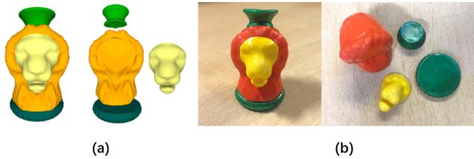
Fig. 1. An example of volume segmentation based on surface attributes. (a) The surface of the model with color attributes, and its segmented volumetric parts using our method. (b) The fabricated result and its assemblable parts.
