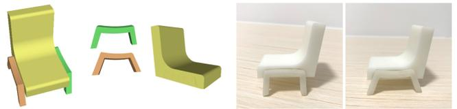
Fig. 17. An example of multi-material fabrication. The chair legs are fabricated by flexible material that can be deformed to different shape.
